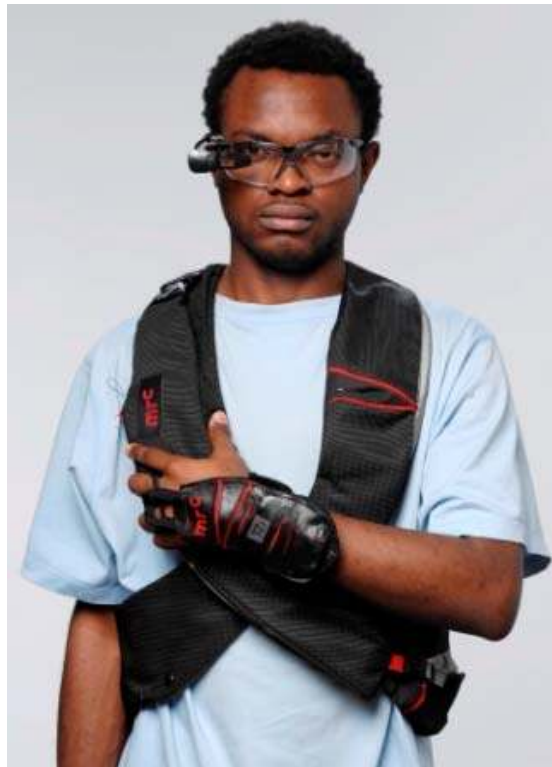
Figure 2: Vest and interaction glove for aircraft maintenance
