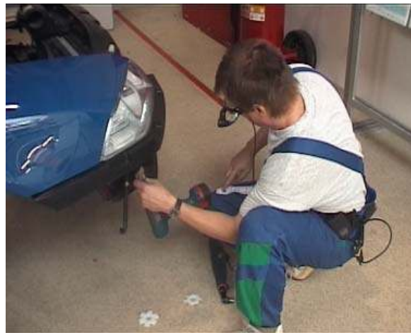
Figure 2: Trainee mounting the headlight by using the wearable computer
