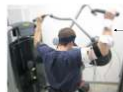
4 randomly placed accel/gyro sensors
