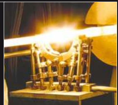
Burner heating preform in lathe
