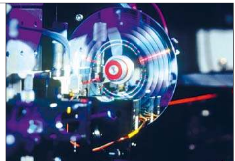
Manufacture of a master compact disc
