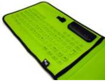
Fig. 70 A prototype ElekTex ® keyboard sleeve for Microsoft's Ultra-Portable computer [134]
