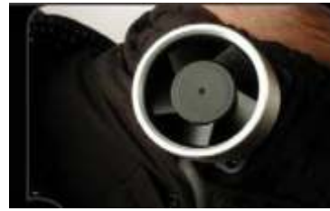
Cooling fan of the heating and cooling jacket
