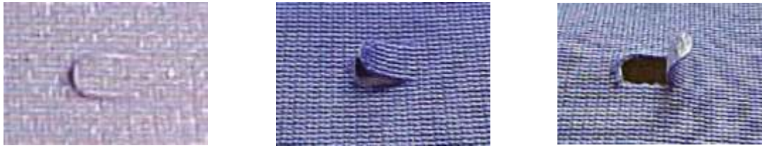
Fig. 110 Flap opening in the textile structure [195]
