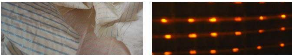
Fig. 63 Inner layer of the energy curtain with integrated reflective and afterglow materials
