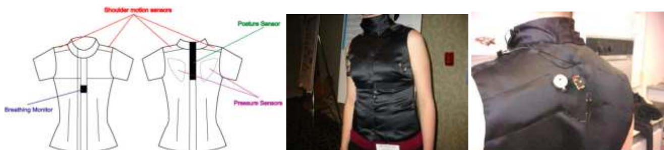
Fig. 50 Schematic presentation and photographs of the foam-based pressure sensor integrated into a garment structure designed by Lucy Dunne
