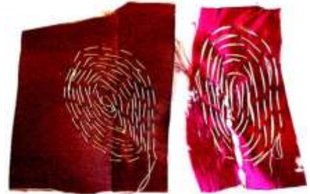
Samples of embroidered rain sensors. The sensors are embroidered directly onto the body fabric and detect contact with water anywhere on the embroidered area
