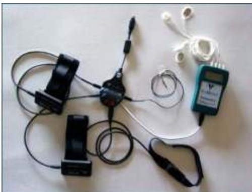
Fig. 45 Optional Serial Expansion Module (SEM) of the Lifeshirt
