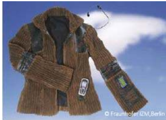
Fig. 25 Communications jacket with textile pad [69]
