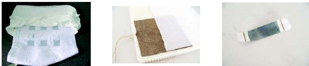
Fig. 68 Textile sensors used in the bed cover [131]
