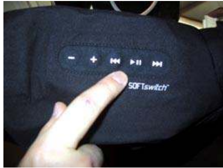
Fig. 9 SOFTswitch™ fabric integrated in the sleeve of a jacket [37]
