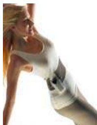
Fig. 44 Conductive fabric area of the warmX ® -undershirt [104]
